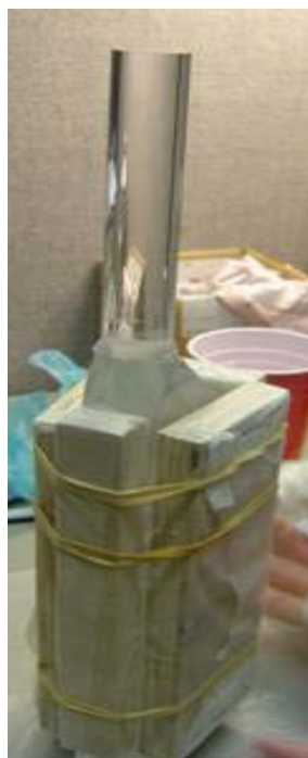
FIG. 8. Making the joint between a block scintillator and its light-guide.
