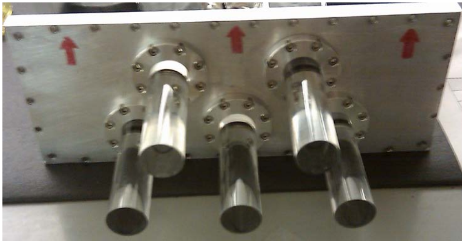
FIG. 7. Plate and Holders support each block scintillator and its light guides.
